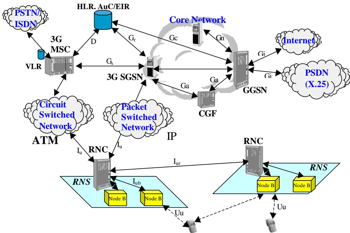
Figure 4 shows protocols used in Node B, RNC and mobile handsets.
