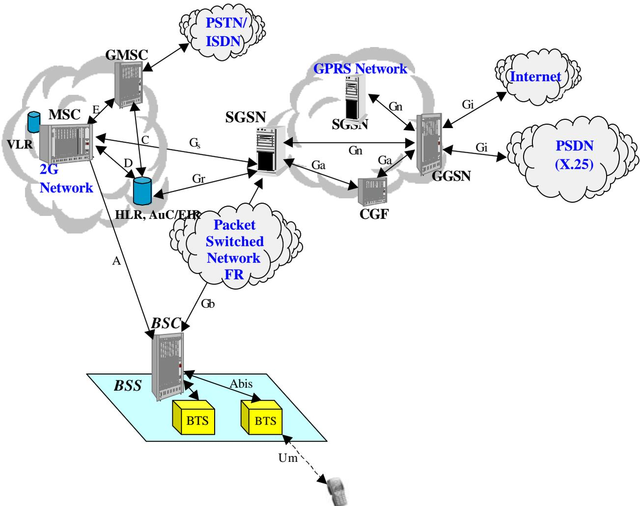
Figure 2 shows the protocols used in BTS, BSC, SGSN, GGSN, and mobile handsets:
